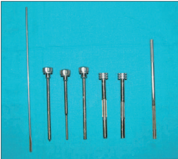
Fig. 1. Surgical instruments originally designed for autologous chondrocyte implantation and then adapted for bone marrow-derived cell transplantation.
